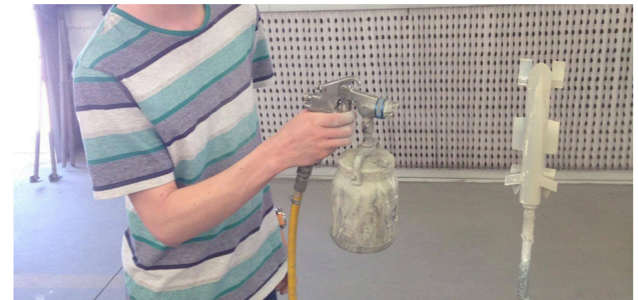
FIGURE 26: APPLICATION OF FINAL COAT
